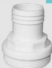
ABS Quick-connect adaptor (2 1/2" - 1 1/2 UN 2A) male thread x 1 1/2" barbed
