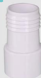
ABS SCH 40 Adaptor 1 1/2" glued male insert (SPIG) x 1 1/2" barbed
