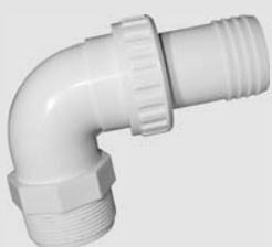
ABS Quick-connect 90° elbow 1 1/2" male thread (NPT) x 1 1/2" barbed
