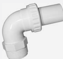
ABS Quick-connect 90° elbow 1 1/2" male thread (NPT) x 1 1/2" smooth
